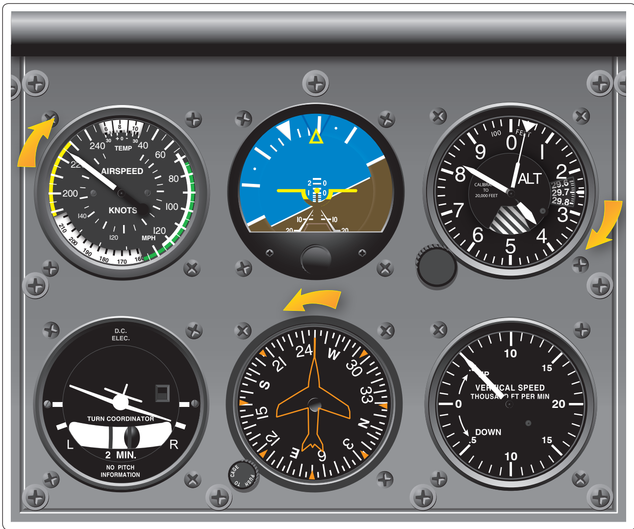
FIGURE 146.—Instrument Sequence (System Failed).
