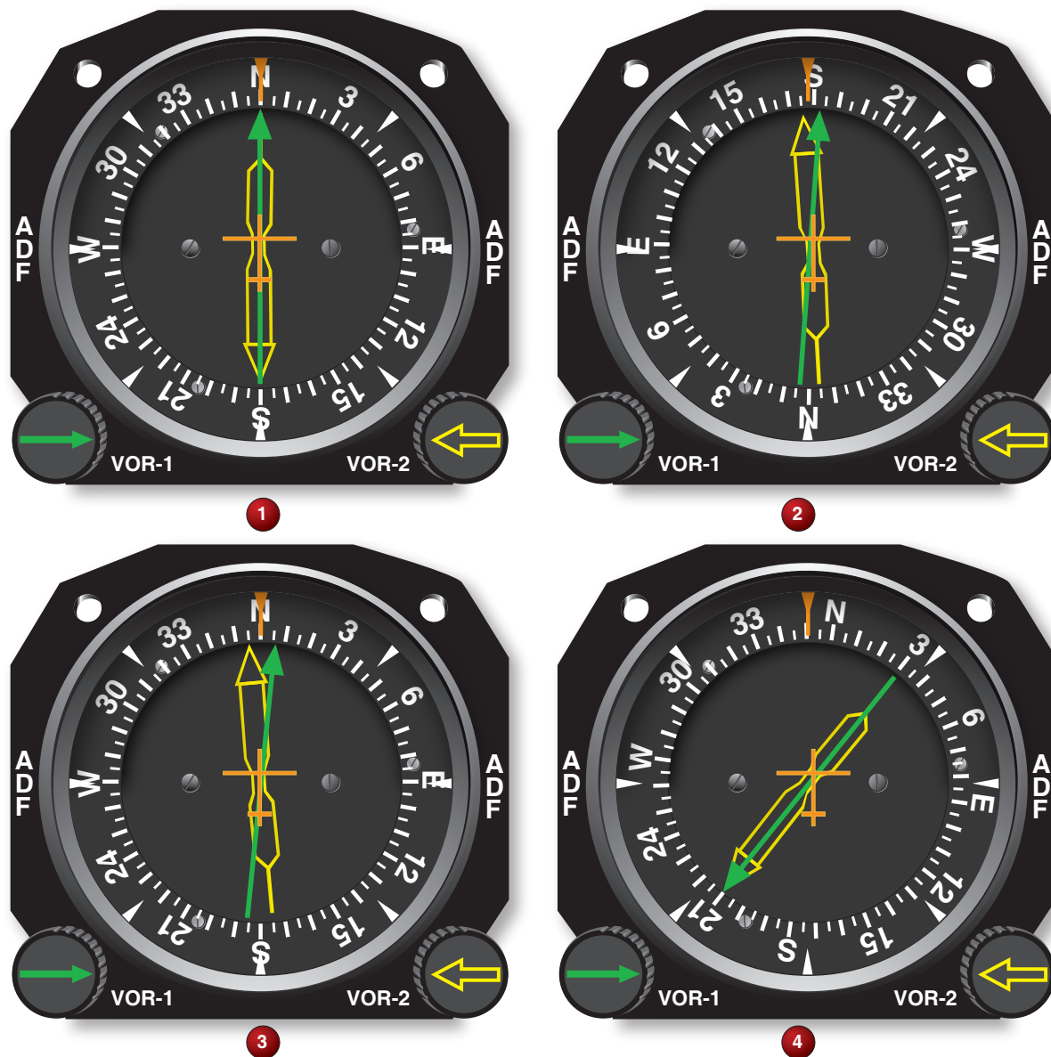
FIGURE 82.—Dual VOR System, Accuracy Check.
